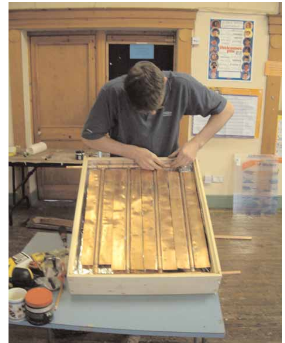
Displaying the copper pipework matrix and copper fins from the interior of the d.i.y solar water heaters.
