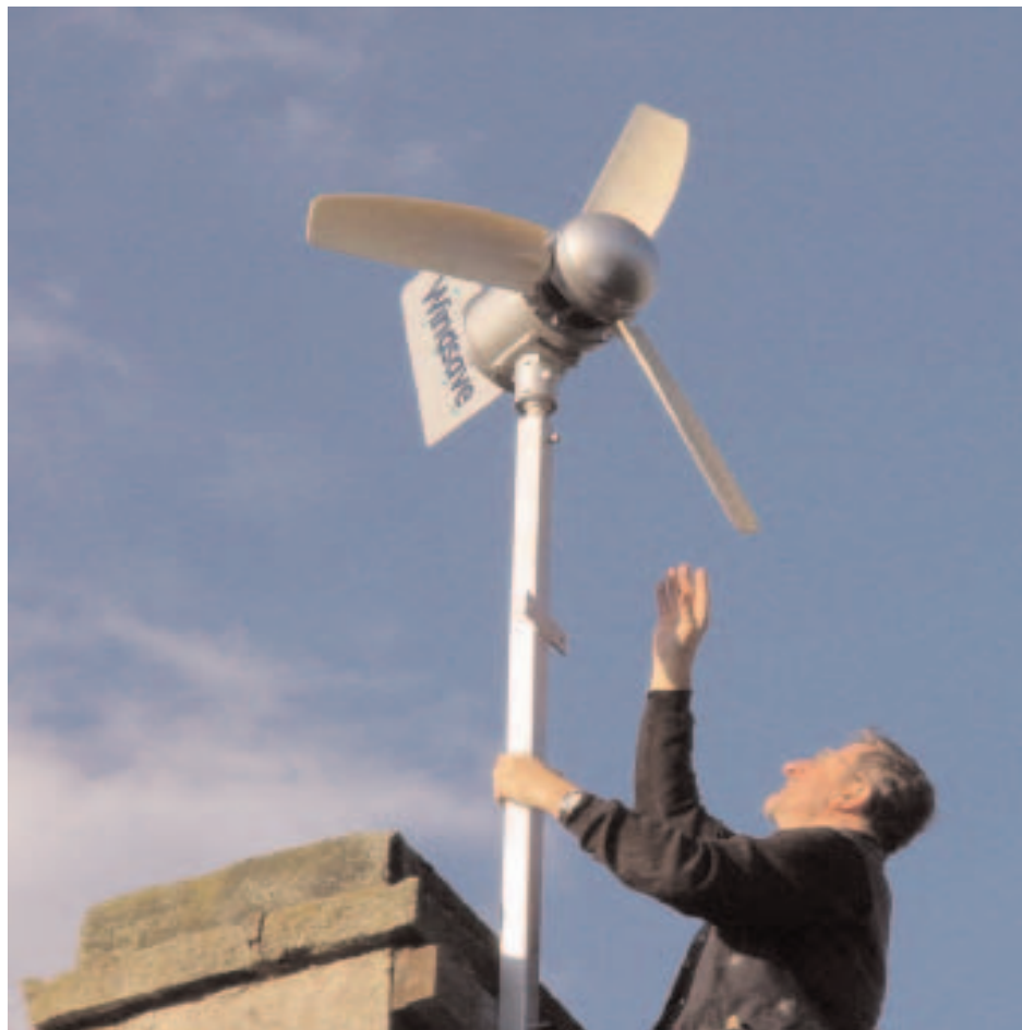
Windsave's pioneering wind turbine designed for use on most urban dwellings.
